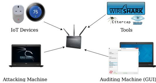
Fig. 2. IoT testbed components
